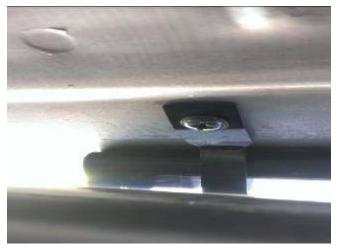
**Step 4-** Now that the bar is installed beneath the vehicle you can start to route the wiring up towards your parking/turn signals. You will want to pull back your fender liner to route the wires into the engine compartment. The following is the color code for the 3 and 4 function side cab lights.
