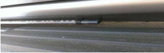
**Step 3-** Next you will use the supplied screws. The screws get screwed into the flat metal surface below the door.
