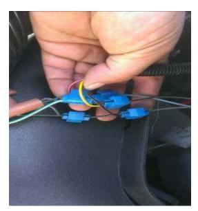
**Step 7-** Once you have the wires all spliced in you can test them to make sure they are working properly by turning on your running lights then your turn signal and then hazards. Once you have tested all the functions you can put your light back in the vehicle and proceed to the other side.
