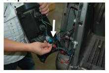
Connect the solid black wire from the light bar to the black ground wire from the tail light using the wire splice connector
