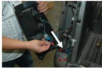
Connect the red wire plus the white and black striped wire from the light bar to the red wire parking light from the tail light using the wire splice connector
