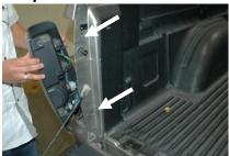
Remove any one side of the tail light housing by removing the two 10mm screws or the two phillips screws depending on the model of your vehicle
