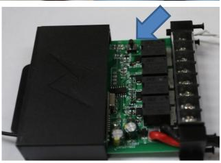
With our earlier models, you will have to open the module by unscrewing the four Phillips screws located by the power connections. With the module energized press the program button located on the upper center of the circuit board and program remote control. Once confirmed that the remote control is working with the module, disconnect fuse and tighten the four Phillips screws securing the case to the module housing.
