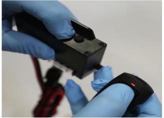
Connect the 4 Channel Remote Control Module to 12 volts. Once the Remote Control Module is energized press the program button on the back of the module. Then press the number 1 button on the remote control. Pairing should take less than 10 second to activate. Cycle through 1-4 to ensure that all channels are response via the remote control. You could pair up to 3 remote controls.
