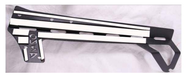
JEEP TJ - THE WHITE LINES ON THE BRACKET INDICATE THE PLACEMENT OF THE FOAM PADS.
