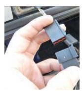
Step 5: Plug in the r third brake light into wire harness.
