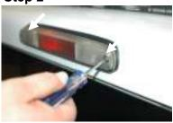
Remove the two phillips screws from the OEM third brake light housing.
