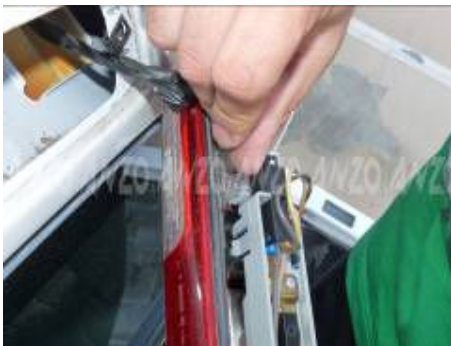
Step 3: Locate the wire harness and unplug it from the light.
