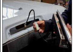
Connect main harness connector from vehicle side to Anzo USA 3rd brake light connector.
