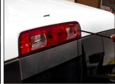
Use Phillip's head screwdriver to remove 2 screws holding factory 3rd brake light in place.
