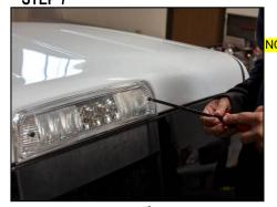
Insert Anzo USA 3<sup>rd</sup> brake light onto vehicle and screw factory screws into vehicle.
