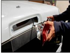
Remove factory 3<sup>rd</sup> brake light from vehicle.
