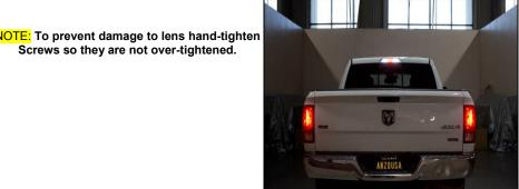
Test cargo and brake light functions on light before operating vehicle.
