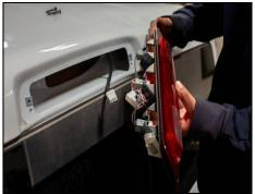
Disconnect main harness connector from factory 3<sup>rd</sup> brake light.
