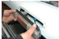
Carefully pull out the OEM third brake light housing from the vehicle.
