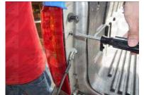
Step 3: Use the phillips screwdriver to remove the two screws holding in the tail light.
