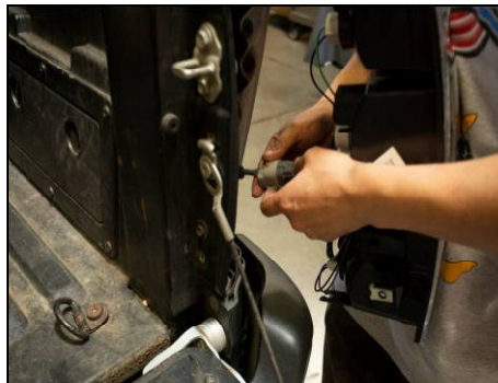
Disconnect main tail light harness connector.
