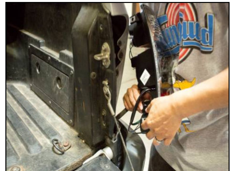
Connect Anzo USA tail light connector to main harness on vehicle.
