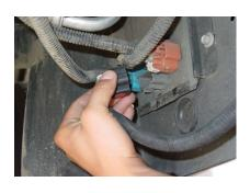
Step 9: Plug the wire harness into the circuit board and test the function of the light to make sure it is working properly
