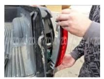
Step 5: Plug in the tail light wire harness into the new Anzo tail light.
