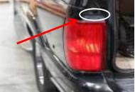
Remove 2 7mm trox wrench screws located on the top of the tail
