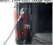
Step 1: Locate the two t27 screws and remove them.
