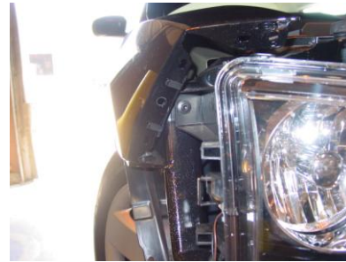
Step 12: Use the T27 torx to remove the outer corner bolt.
