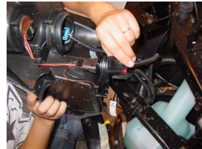
Step 16: Unplug the main wire harness.
