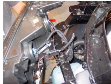
Step 15: Remove the original headlight from the vehicle.
