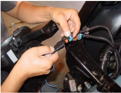
Step 20: Strip back loose black wires and splice into the black wire going into the headlight.
