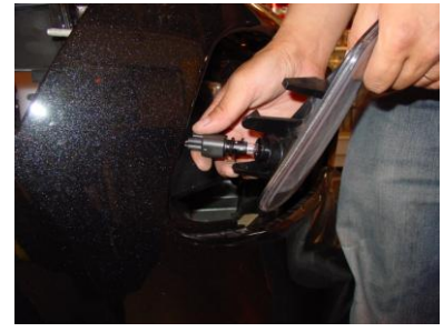
Step 10: Remove the corner light bulb from the assembly.
