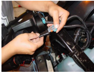
Step 21: Strip back loose blue wires and splice into the red wire going into the headlight.
