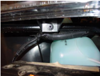
Step 14: Remove the bottom bolt on the headlight unit.
