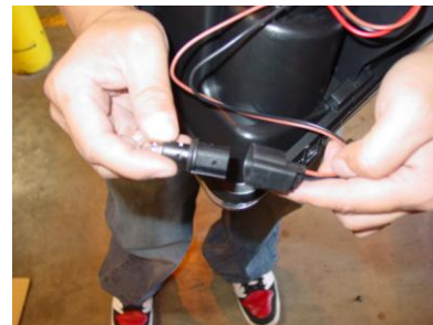
Step 18: Remove the corner light bulb assembly.
