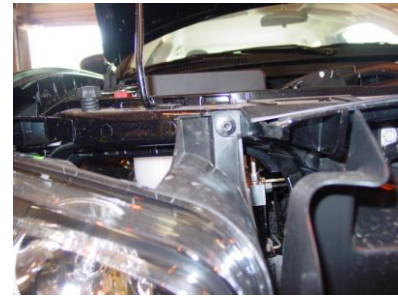
Step 13: Use the T27 torx to remove the inner corner bolt.
