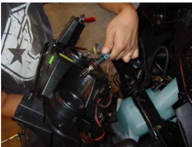
Step 17: Remove the high and low beam connectors.
