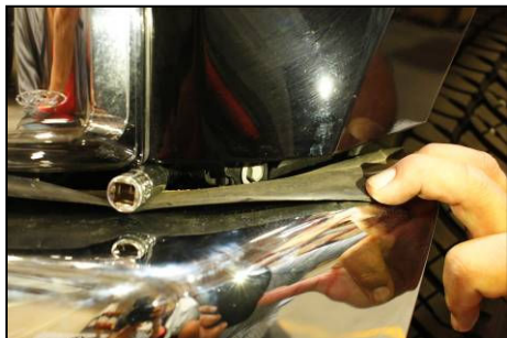
Remove lower outer 10mm fender headlight bolt behind rubber bumper molding
