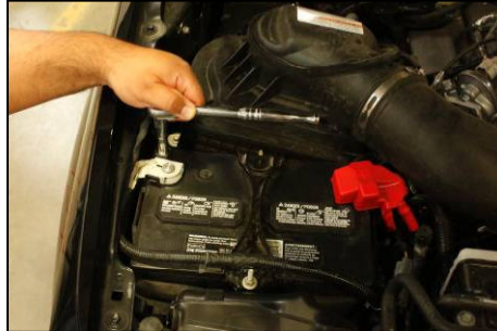
Open hood and disconnect negative battery terminal
