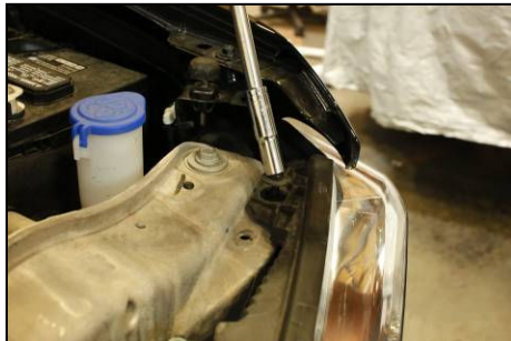
Remove top 10mm headlight bolt
