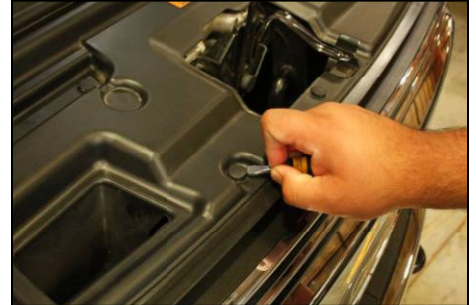
Remove 13 body panel clips from radiator shroud
