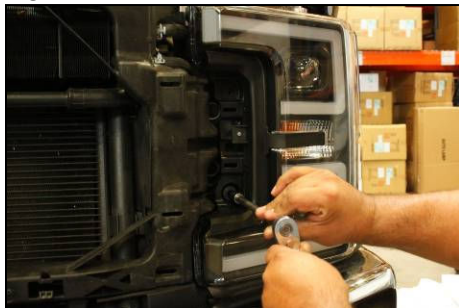
Reverse steps 9-12 to install new Anzo USA headlight
