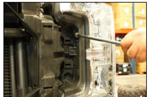
Remove two 10mm inner headlight bolts
