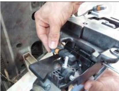
Step 13: Plug in the wire harness socket for the new Anzo head light.
