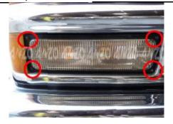
Step 1: Remove the four phillips screw holding in the parking light.
