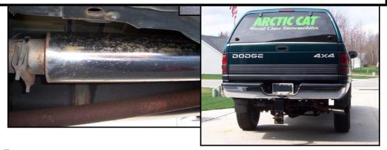
There *are* differences—and they should be factored into the decision when purchasing an <u>exhaust system</u>. The four main variables include: **corrosion resistance, temperature endurance, finishing quality and price.**
