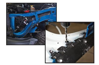
8. Place carbon fiber vent on fender and reuse the (3) plastic pushpin retainers and new rivets to fasten in the OE location.
