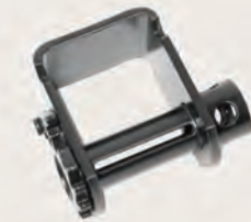
43565-127 Web Storable C Track Slider. Lighter 7mm heat treated frame Weight: 8.2 lbs./3.7 kg. WLL: 6,000 lbs./2,730 kg.
