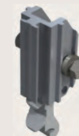
50187-31 Lift-A-Deck II Low Profile Foot Assembly. Machined guide shoe allows for inspection of both locking lugs while beam remains installed in the track. Features a coil spring for optimum service life. Weight: 0.6 lbs./0.27 kg.
