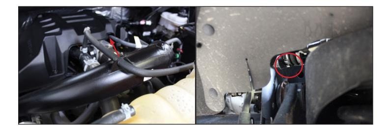
10) Unclip the coolant expansion tank line from the right-side intake tube and from the right front wheel well, use a long screwdriver or 7mm socket with extensions to loosen the hose clamp on the right tube that connects it to the turbo inlet.
