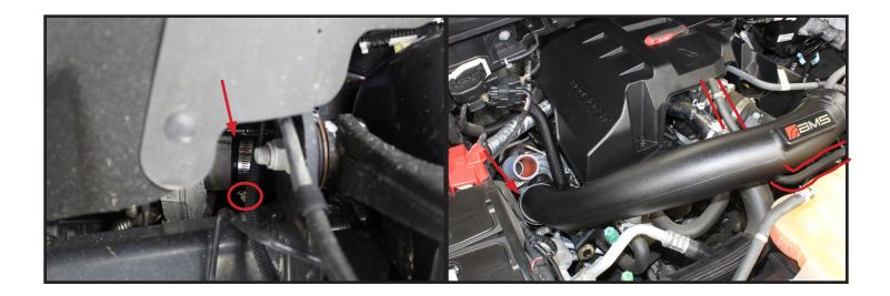
16) Ensure the silicone is fully seated onto the turbo inlet and tighten the hose clamp. Once the tube stanchion is fully seated in the rubber grommet and the tube is properly aligned, tighten the larger hose clamp to the same tightness as specified for the left tube. Make sure the expansion tank hose is routed underneath the tube.
