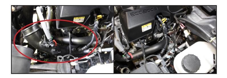
6) Remove the left side OEM inlet tube from engine bay.
