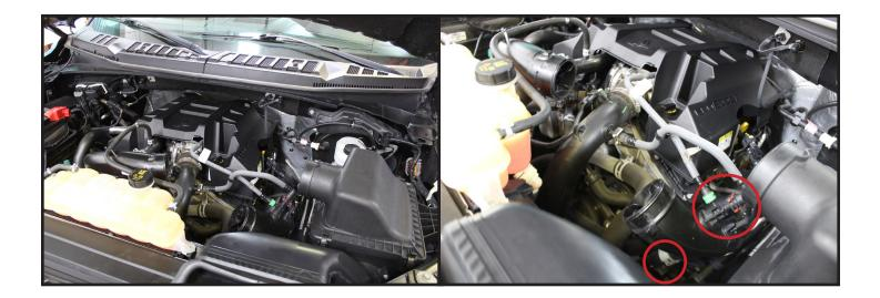
2) Remove the y-pipe and set aside. Next, the connections to the fittings on the left side inlet tube must be disconnected.
