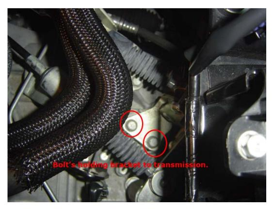
4. Remove the black plastic cap from the bracket and remove the 12mm nut, lock washer and flat washer.
