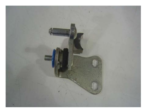
5. Separate the arm and bracket and remove the oem plastic bushings.
