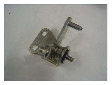
8. Install plastic bushing on other side as shown below then follow up with the washers and 12mm nut then finally the black cap.
