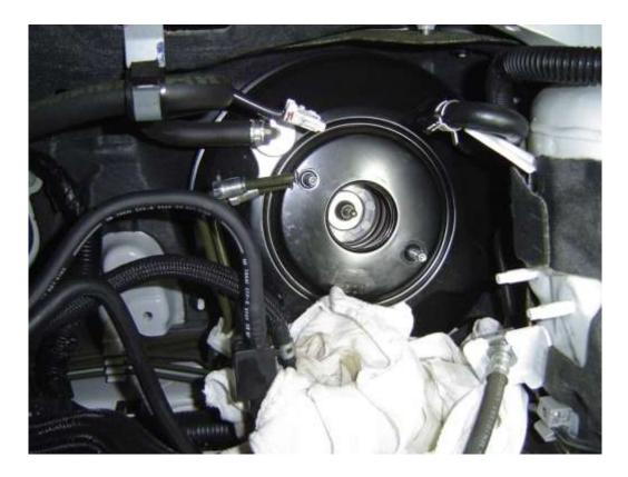
3. At this point you can remove the brake booster. Begin under the dash and remove the 4 nuts holding it to the firewall. And then remove the clip and pin holding it to the brake pedal. While under here pull the clutch master cylinder shaft off of the clutch pedal also.
