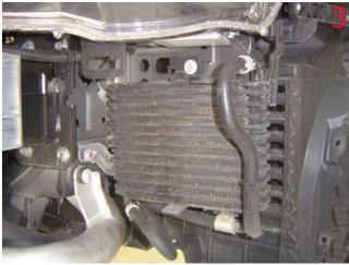
5. Place a clean container under the transmission cooler <sup>4</sup>, disconnect lines and let them drain into the pan. You MUST catch all fluid and put it back into the transmission when done, there is no way to measure the fluid level in the transmission. You can now also remove the transmission cooler and drain all of the fluid from it into the pan also, make sure not to get any dirt or debris
