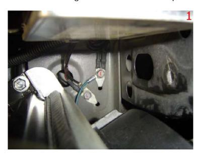
2. Connect the blade connector to one end of the fuse holder and the red wire to the other end using the supplied butt connector. Connect the blade connector to the terminal as shown  $^2$ . Run the wire out of the box to the side of the grommet  $^3$ .
