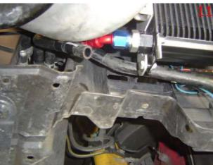
10. Now remove the cooler from the car and push the fittings onto the hose and clamp tightly <sup>12</sup>. The fittings fit very tightly into the hose, heating the hose up helps it to expand and fit over the fittings, a little transmission fluid on the barbs will also help the fittings slide in easier. The 120 degree fitting goes on the longer/top hose, the 45 degree fitting goes on the shorter/lower hose.
