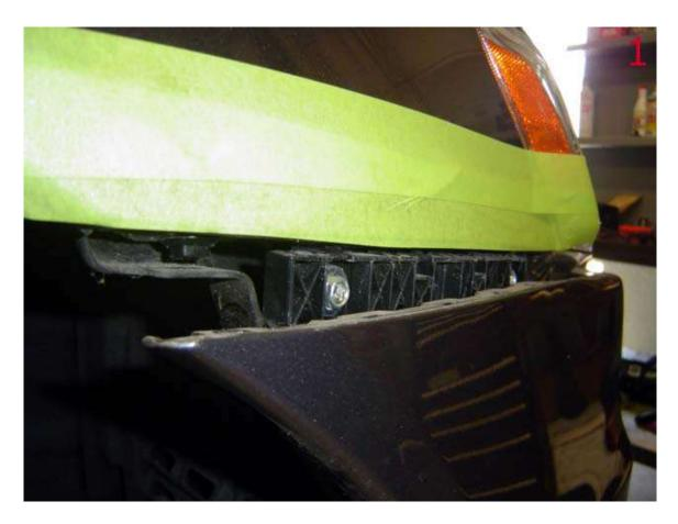
4. Remove the factory transmission cooler duct, it is held on by 3 clips  $^{2,3}$ .
