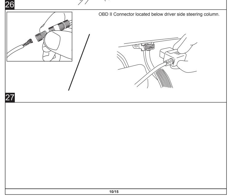
**OBD II install:** Use Supplied Posi Twist connectors to attach the Plug and Play Module to the Harness. Attach matching colors on the harness to the wires on the module. Plug in module to OBD II port on the vehicle. Secure harness with supplied tie wraps.
