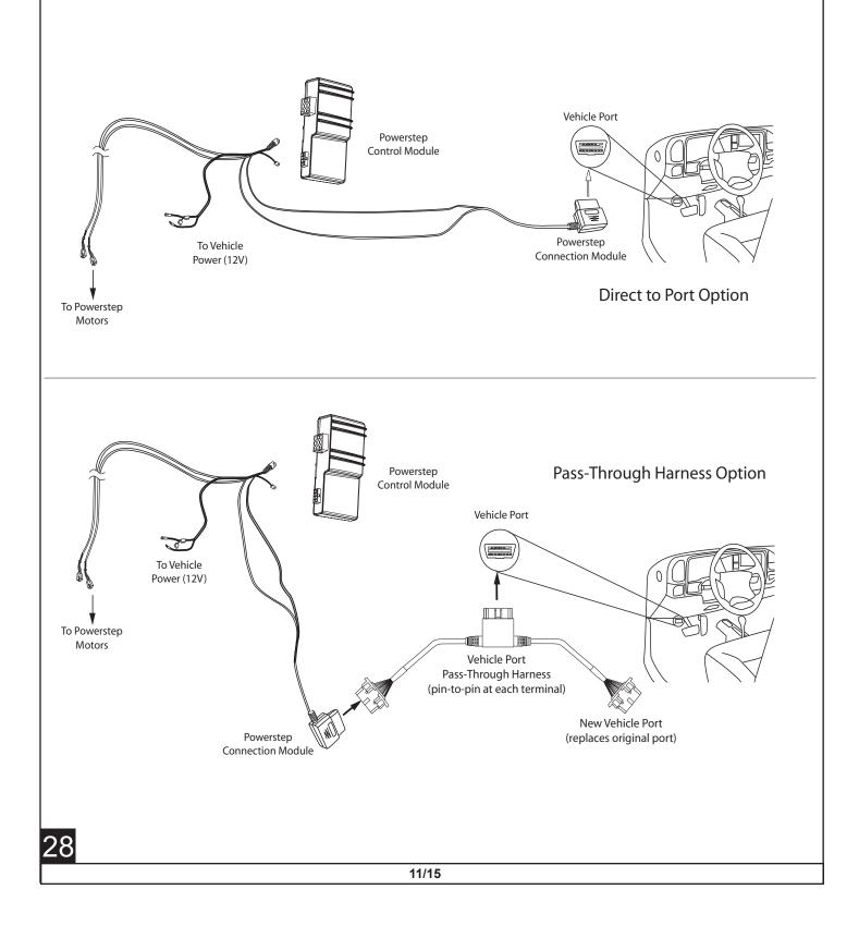
Route the two Wire Harness legs down over the wheel wells toward Motor Linkages, long leg across to the passenger side. Secure harness with tie wraps.
