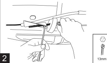
Remove brake cable guide from frame by depressing locking tabs and sliding guide out through hole. Unthread brake cable from frame mount.
