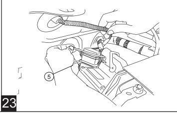
Connect power leads from Controller, Red to positive battery terminal and Black to the vehicle body ground as shown.
