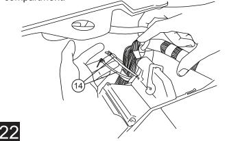
Remove fuse from Power Step Wire Harness.
