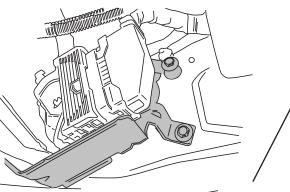
While holding brake cable adjustment nut with wrench (located on driverside along frame, towards the rear), loosen brake cable to allow for slack. Mark position of nut before loosening.
