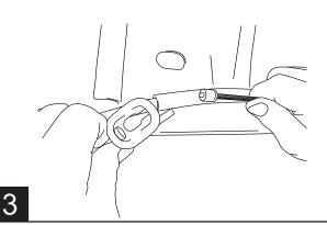
Attach brake cable guide to supplied Brake Cable Bracket (27) and mount bracket with supplied hardware. Reattach brake cable and readjust brake cable adjustment nut to original position.
