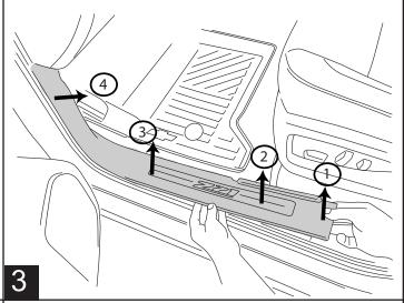
Pull up the carpet and drill 9/32" hole in metal and insert supplied rubber grommet (21).
