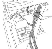
Remove power fuse. Attach power lead (RED wire) to positive pole on the battery. Attach ground lead to negative battery pole.
