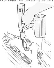
Route wire harness along the frame and back towards rear linkages. Secure with zip ties. Push both wires through rubber grommets.
