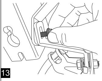
Set step pad into center position and tighten screws. Tighten to 5 ft-lbs.
