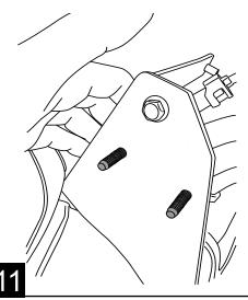
Set frame mount into position and tighten two bolts.
