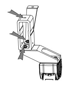
Using a 15mm socket with extension, align bolt with threaded plate. Do not tighten.
