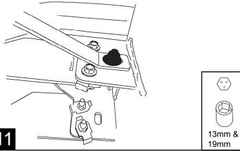
For all other Models: Attach bracket to threaded hole in frame mount. Rotate bracket into position and use the provided M12 hardware.
