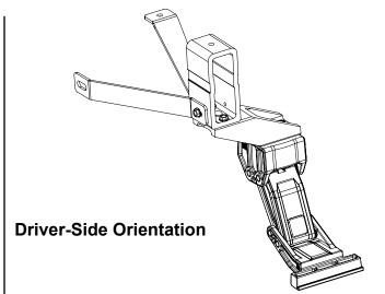
Using a 15mm Socket assemble Lateral mount onto Linkage assembly. Torque bolts to 20 ft-lbs. Note: Drivers side shown. Mirror for passenger side.
