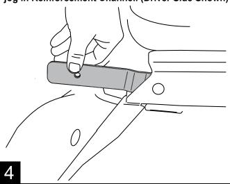
Locate the step pad on the center position of the lower linkage assembly and secure using provided PT Screws. Tighten to 5 ft-lbs using T25 Torx bit. Align Step pad to be in line with fender.
