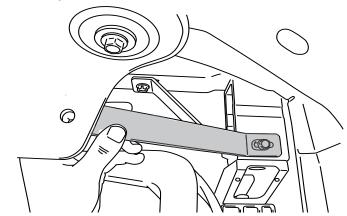
NOTE:If a hole is not provided on a factory body mount, a hole must be drilled using a 1/2" drill bit.
