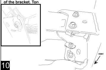
For 2011 - up Short bed models: Attach bracket to threaded hole in frame mount. Rotate bracket up to position and use provided M12 Hardware. Tighten M8 bolt to 16 ft-lbs and M12 bolt to 35 ft-lbs.
