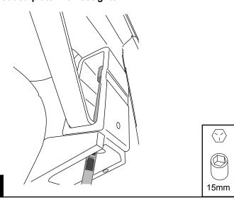
Using a 15mm socket with extension, align bolt with threaded plate. Torque to 20 ft-lbs.
