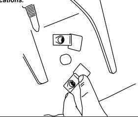
Offset the step pad forward and secure using provided PT Screws. Tighten to 5 ft-lbs using T25 torx bit. *Note: Drivers side shown*
