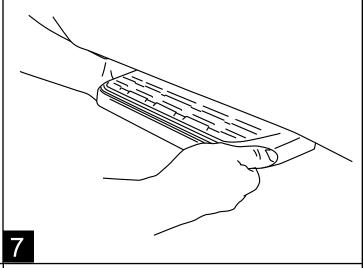
To retract, gently kick up on the underside of the step pad.
