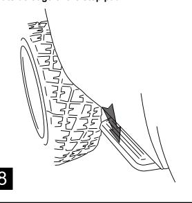
Set linkage in place and tighten bolts using a 15mm socket. Torque bolts to 20 ft-lbs.
