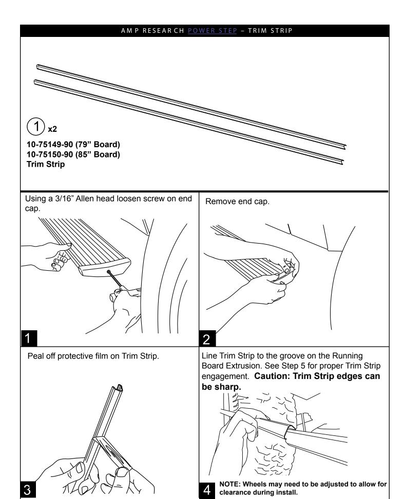
NOTE: Trim Strip should be lined up in both the upper and lower grooves.
