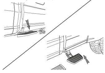
To retract, gently kick up on the underside of the step pad.
