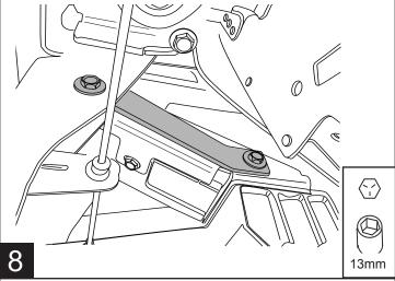
Remove bracket and pre drill hole using a 1/8" drill bit then drill to 3/8".
