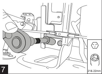
Attach rearward support bracket (#6) using supplied M8 hardware (#8) Bolts and (#9) Nuts. Locate bracket as shown. Center punch hole using bracket as a guide as shown.
