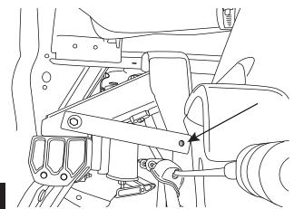
Install rearward support bracket (#6) using supplied M8 Hardware(#8) Bolts and (#9) Nuts. Torque to 16Ft-Lbs.
