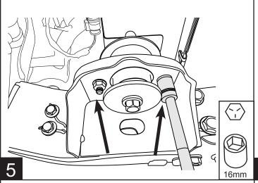
Using a 21mm socket and wrench remove Lower tow hook bolt. Loosen upper bolt enough to slide bracket up into position.
