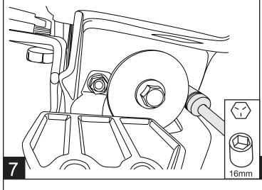
Use supplied bolt(6) and washer(7) for lower tow hook bolt that was removed in step 6. Snug bolts but don't tighten.
