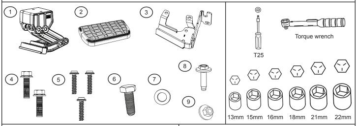
Using a 15mm wrench assemble steel bracket to Linkage assembly. Torque bolts to 20 ft-lbs.
