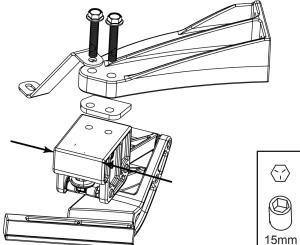
Remove corner bumper cap and use flat blade screwdriver to pry loose. Use caution when removing tabs.
