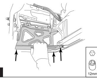
Replace Re enforcement bracket. Reinstall bolts from step 6 and 7. Use provided nuts to secure bracket in place. Replace bumper components from steps 2-5.
