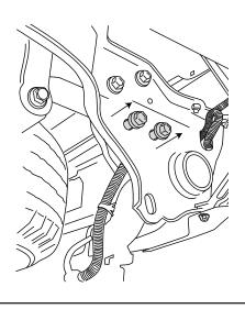
Install mounting bracket using factory fasteners. Torque fasteners to 90ft-lbs/125Nm. Align bumper support bracket to mounting hole in Re enforcement bracket. Torque nuts to 33ft-lbs/44Nm.
