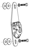
Passenger side, Bracket and hardware orientation
