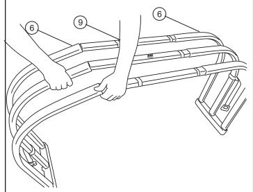
Slide 3 center tubes into the open ends of the bent tubes as shown. Insert center tube with logo into the center tube.
