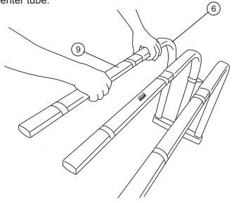
Adjust the width of the BEDXTENDER by placing the pivots into the mounting brackets. To keep overlap consant, adjust each tube so that the gap between the edge and the tape is the same.
