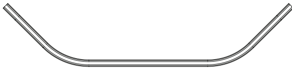
8 Double Bend Center Tube (With AMP Logo)
