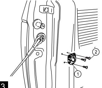
Fasten mounting brackets using the supplied self-tapping Phillips screws and torque to 30 in. lbs. If equipped with a bedliner, install mounting brackets over bedliner.
