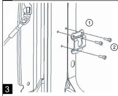
Fasten mounting brackets using the supplied self-tapping Phillips screws and torque to 30 in. lbs. If equipped with a bedliner, install mounting brackets over bedliner.
