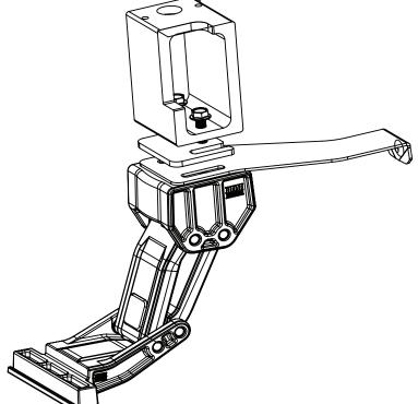
NOTE: Bracket P/N 16-03850-90 and bolts 19-03341-90 from PN 75406-01A will no longer be needed when using this dually upgrade kit.
