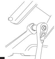
WARNING: Rivet Nuts not properly collapsed will not hold securely to sheet metal.
