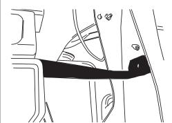
Remove Linkage assembly and center punch hole.
