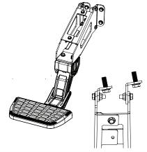
Brackets must be configured for Passenger Side 5 1/2 ft Bed as Shown.
