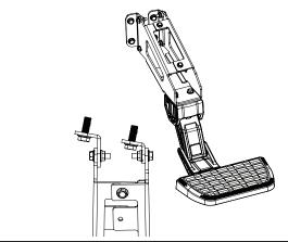
On Driver side, first bolt (3) over (4) and tighten all three (9) M8 Bolts (2 on the top, 1 on the bottom) to 20ft lbs. below as shown. Second, use bolt (8) to bolt (6) to (3) and (5) to (4) to flanged nut (11). Mirror for Passenger Side.
