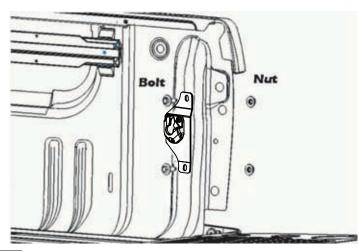
Place Mounting Bracket aligned with top hole. Allow bracket to hang vertically. Mark (Center Punch) location of lower hole using the bracket slot as a template. Remove bracket. Drill hole with 1/8" drill bit then drill out hole with 21/64" drill bit. Use file to remove burrs. Apply primer to edge of hole. Allow primer to dry.
