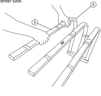
Connect the two halves. Make sure there is at least 3" overlap with the bent tubes on each side.
