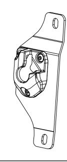
Use the M5 bolts and nuts to fasten the Quick Mount Bracket to the mounting bracket. Apply thread locker to the tip of the M5 bolt. Torque to 8 ft. lbs. Allow 10 minutes to dry before handling. (Passenger side shown)
