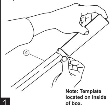
Slide 3 center tubes into the open ends of the bent tubes as shown. Insert center tube with logo into the center tube.
