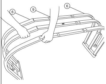
Adjust the width of the BEDXTENDER by placing the pivots into the mounting brackets. To keep overlap consant, adjust each tube so that the gap between the edge and the tape is the same.
