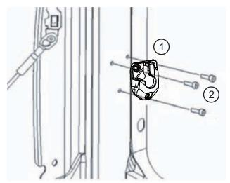
Fasten mounting brackets using the supplied self-tapping Phillips screws and torque to 30 in. lbs. If equipped with a bedliner, install mounting brackets over bedliner.
