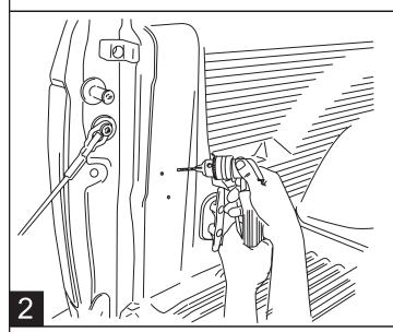
Using a power drill and 9/64" drill bit, drill through the sheet metal. If equipped with a bedliner, drill through bedliner.
