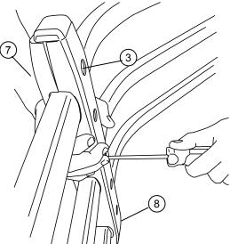
NOTÉ: Do not over tighten as this may strip out. Fastener will reach a noticable stopping point.
