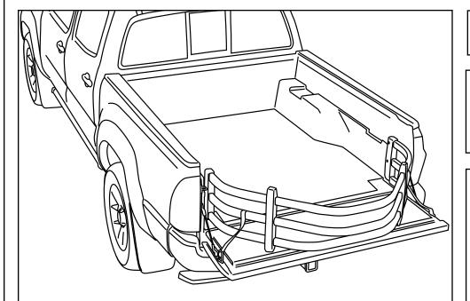
MOTOXTENDER HD™ shown assembled and installed on truck.
