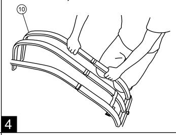
Adjust the width of the MOTOXTENDER to fit the pre-installed mounting brackets. To keep tube overlap constant, adjust each tube so that the gap between the edge and the tape is the same.
