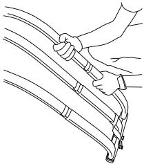
Note: Install Strap Buckle Assembly to center tube of Pivot Upright Assembly.
