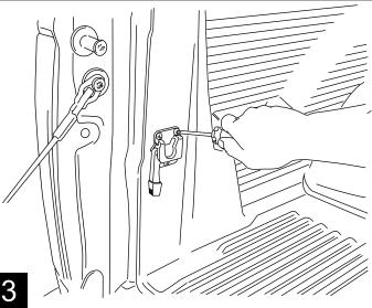
Fasten quick latch mounting brackets using the Phillips head screws and torque to 30 in. lbs. If equipped with bedliner, install quick latch mounting brackets over bedliner.
