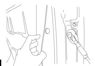
Mark hole position on bedliner for both top and bottom holes and center punch to make a drill guide.
