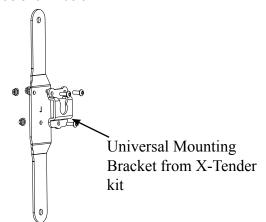
Pass button head bolt through internal tooth washer, mounting bracket and hold down bracket and engage with nut.
