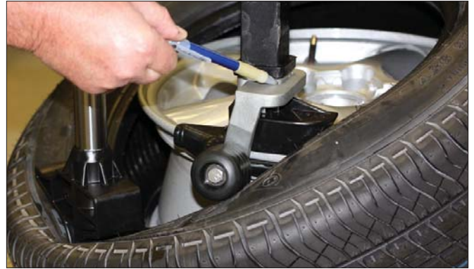
Figure 22 - Duckhead Roller Properly Mounted On Bracket
