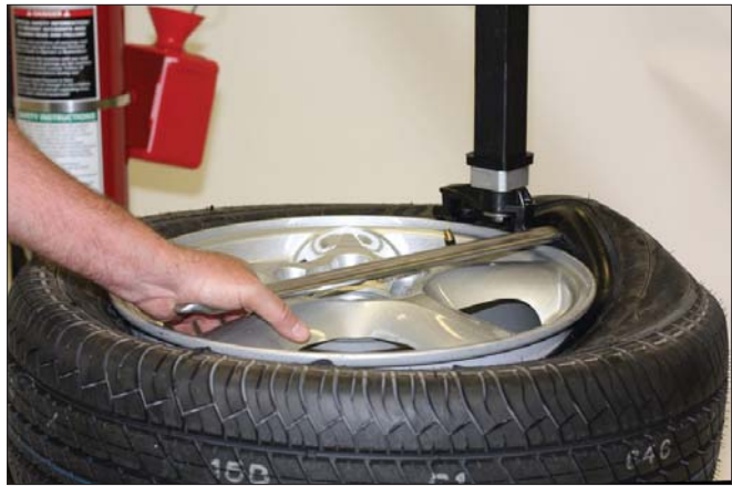
Figure 40 - Rotate Lifting Tool Down for Demount
