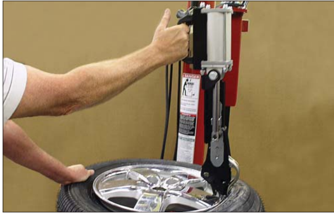
Figure 51 - Leverless Tool Hooked Under Tire Bead
