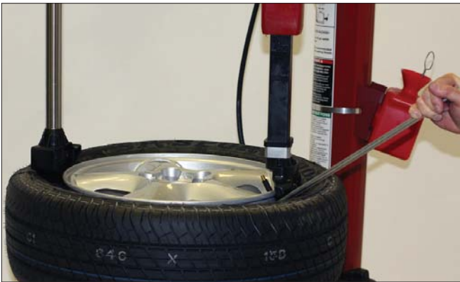
Figure 38 - Helper Foot Pushing Bead Into Drop Center
