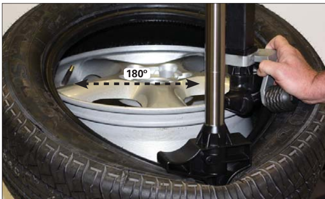
Figure 21 - Position Valve Stem 180° Ahead of Mount Tool
