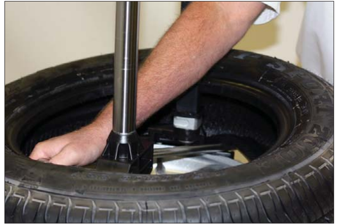
Figure 15 - Guide Lower Bead Over Knob On Demount Tool
