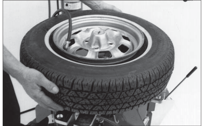
Figure 25 - Lift Tire Upwards for Bead Sealing
