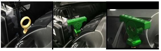
3. Orient the windshield washer cap over the existing cap and press down to snap into place.
