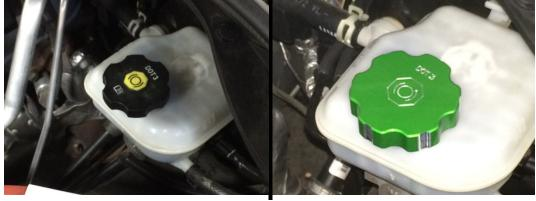
5. Remove the tape backing on the inside of the master cylinder cap. Press the cap over the existing cap and hold down for 2-3 minutes to ensure adhesion.
