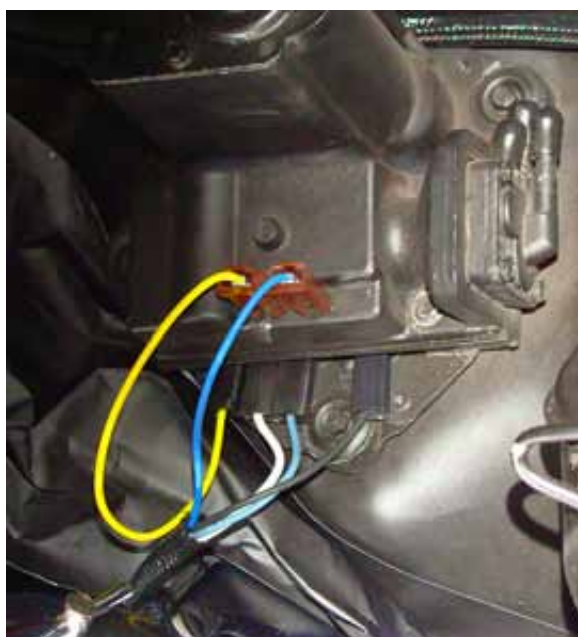
FIGURE #3 WIPER MOTOR CONNECTIONS
